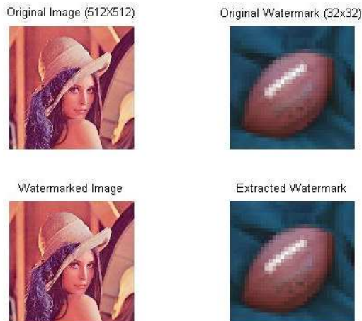
Fig. 2. Original color image, watermark, watermarked image and extracted watermark for algorithm I.
